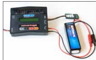
Connection of a battery with external balancing connector
