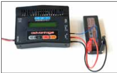
Car battery connection (with SLPB balancing wire)
