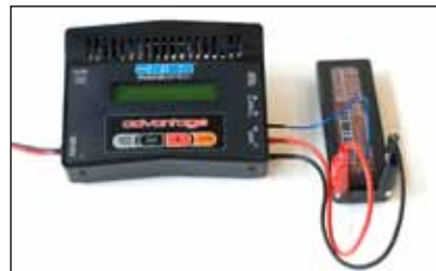
Car battery connection (with SLPB balancing wire)
